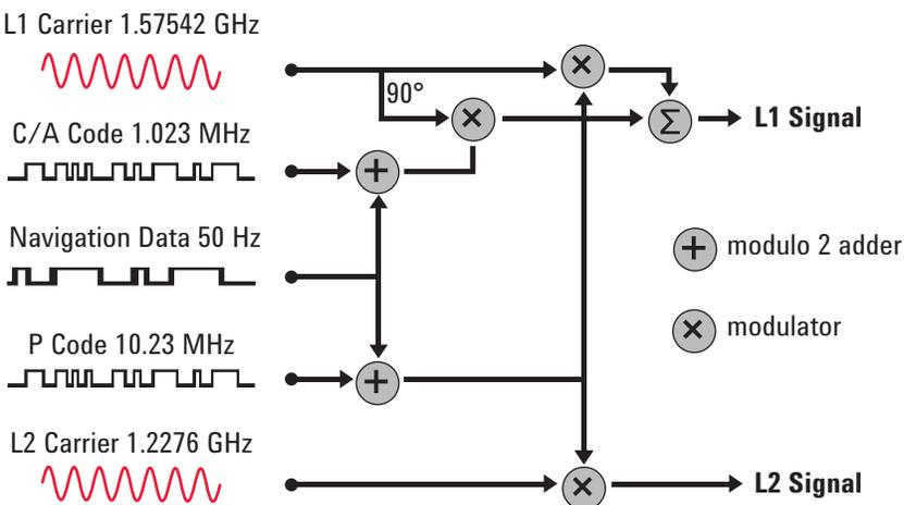
Figure 1. GPS signal structure.
