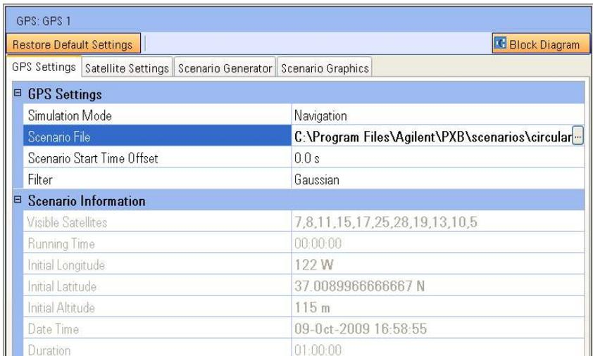
Figure 7. N7609B GPS settings tab.
