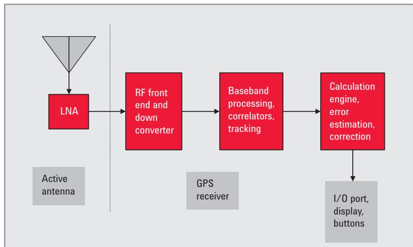
Figure 2. GPS receiver block diagram.
