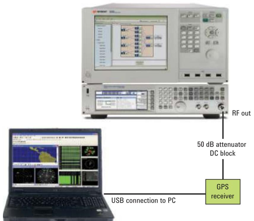
Figure 5. Typical GPS receiver test setup.
