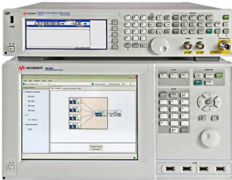
Figure 3. N5106A PXB and N5182A MXG RF signal generator.
